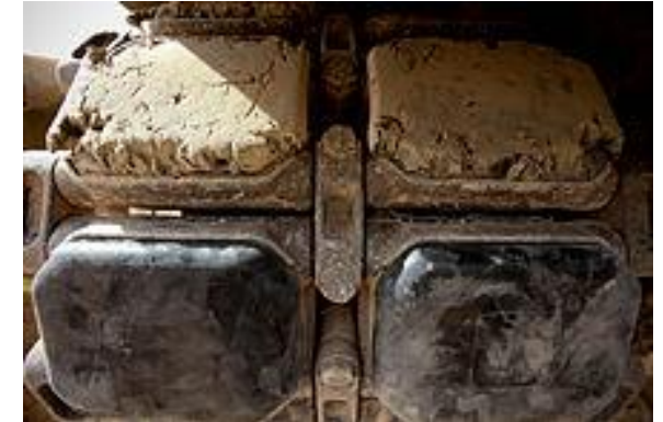
Worn and new track pads on an M1 Abrams battle tank.
