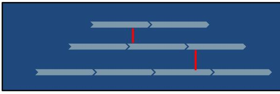
Crosslinking significantly increases the size of an elastomer molecule with a few reactions and prevents movement. Example: Finished Tube
