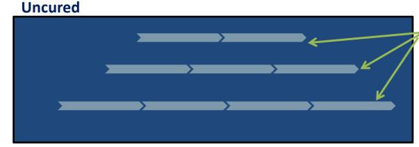
Polymer molecules above the glass transition temperature can move around.
