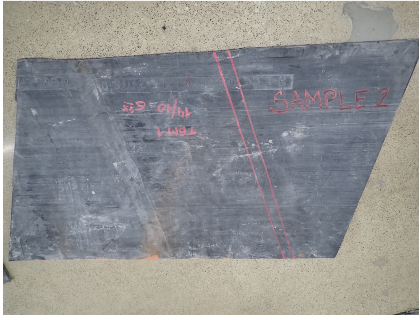
Sample 2-Intact splice from Supplier A
