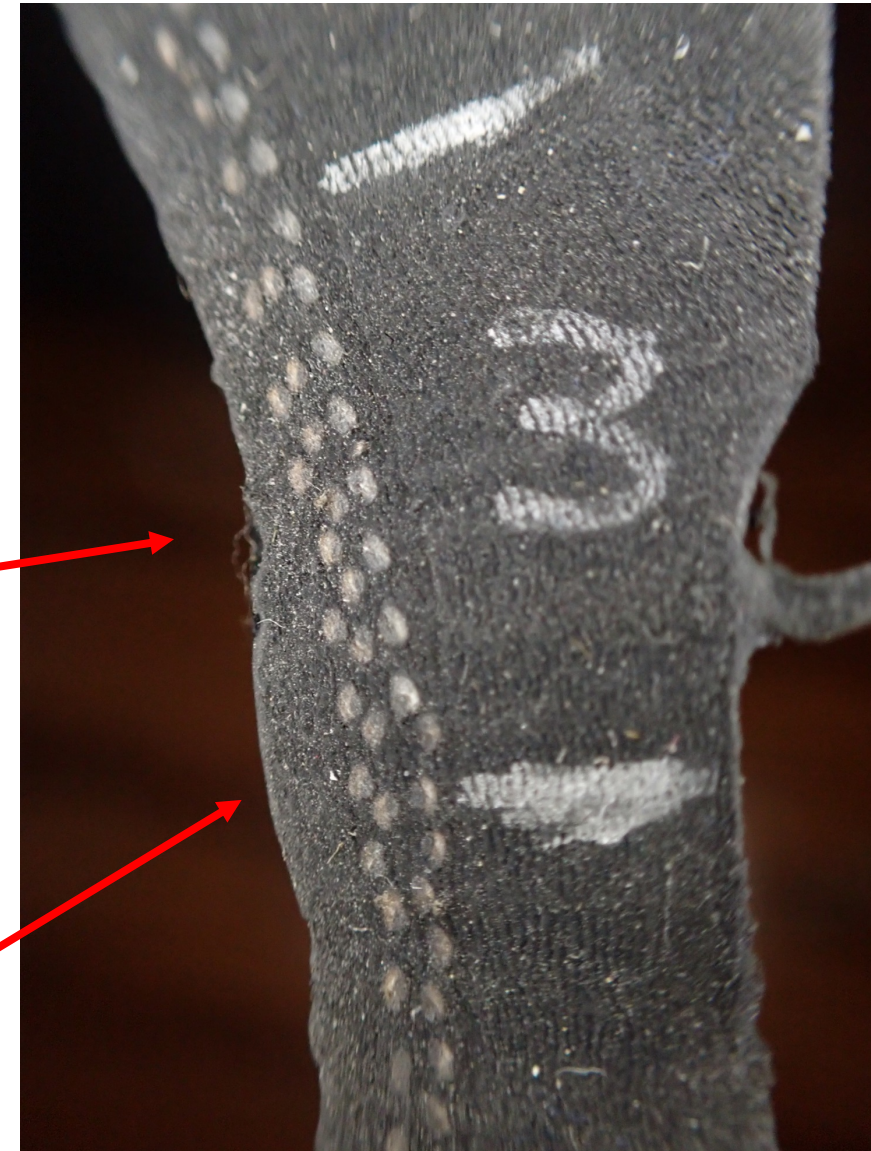
Interface A splice-~8 cord overlap
