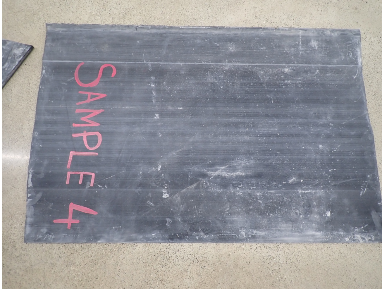
Sample 4-Unspliced control section
