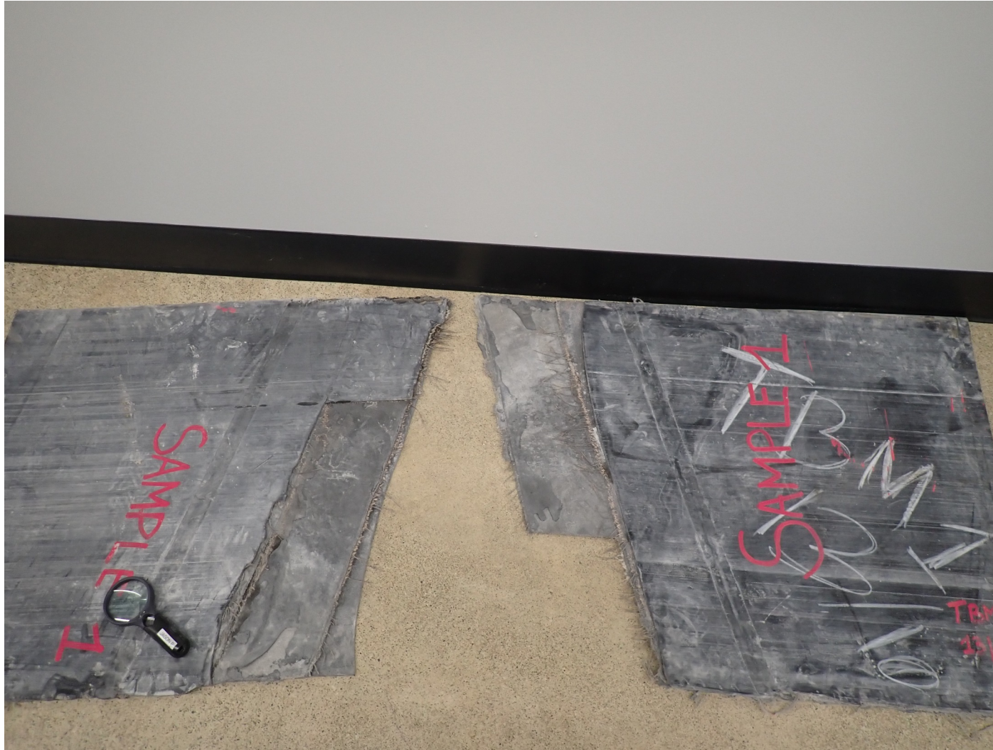
Sample 1-Failed splice from Supplier A
