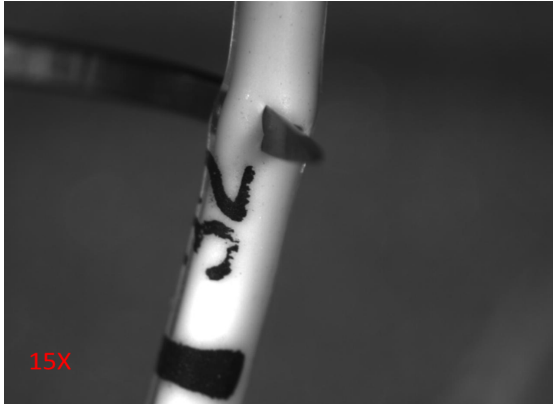
Exemplar catheter punctured with suture needle.
