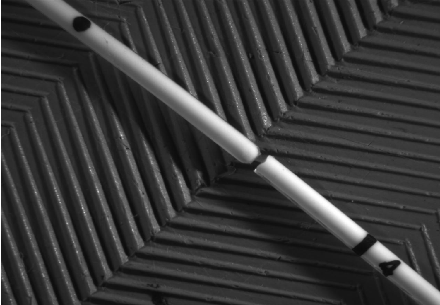
Incident Catheter point of failure, 5X Magnification.
